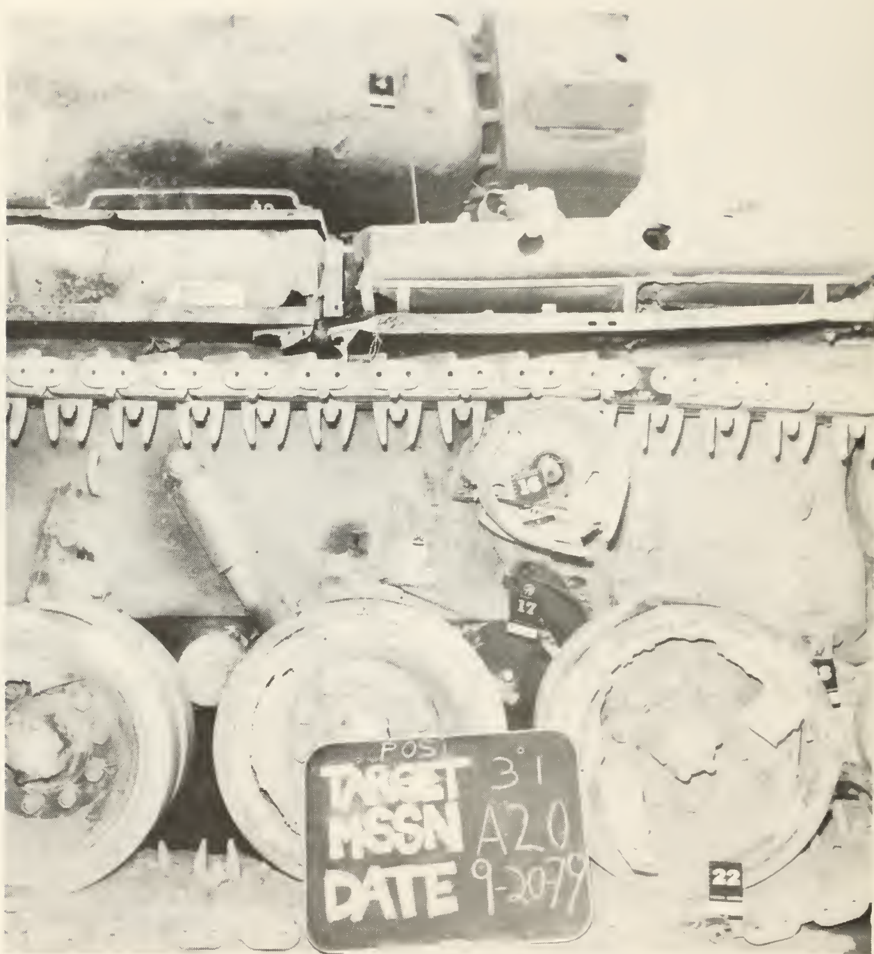
FIGURE 34. Impact 17, Perforation of Hull and Fuel Tank, Tank 31.
